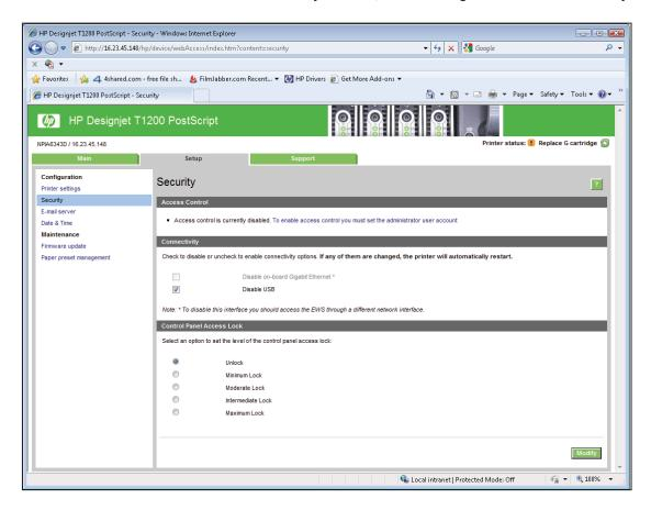
If a connectivity option is enabled or disabled, the printer will automatically restart. Keep in mind that disabling a connectivity option could cut off network access to the printer. As a security measure, disabling the connection used to access the Embedded Web server is not permitted.
