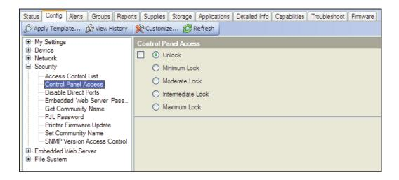
This option can be enabled from the T1200 Embedded Web server as shown below:
